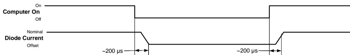
Figure 3 : Computer on-Off function diagram
