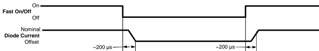
Figure 7: Fast On-Off gate function diagram
