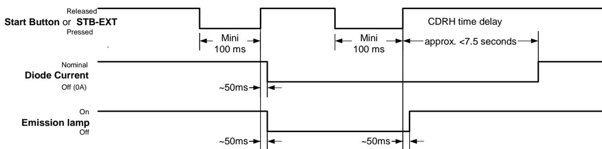
Figure 8: Laser On-Off function diagram (similar to STB-EXT)
