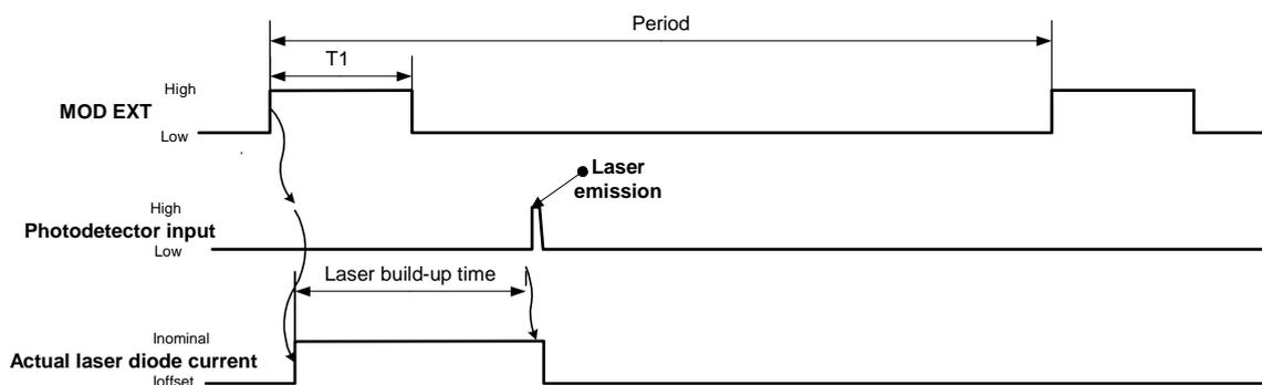
Figure 2 : triggered lasers pulse generation sequence
