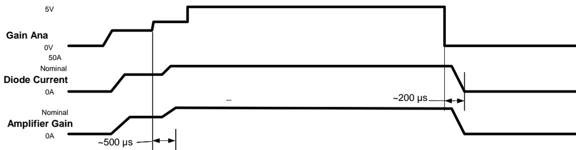
Figure 6: Fast On-Off diagram
