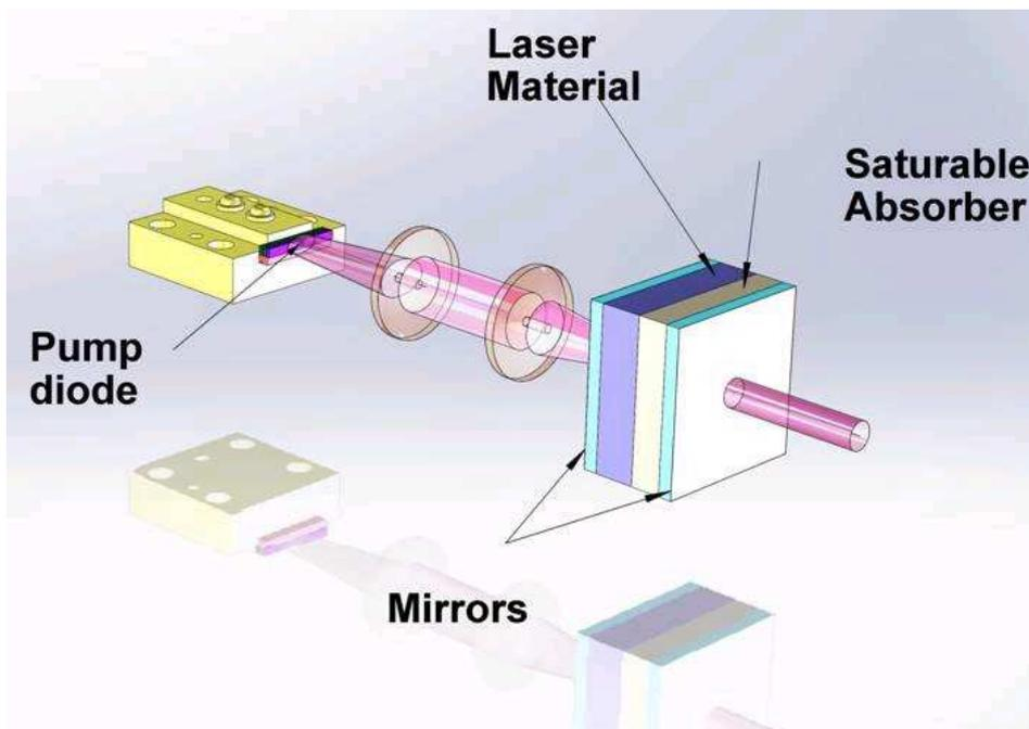
Figure 1: passively Q-switched microchip laser architecture
