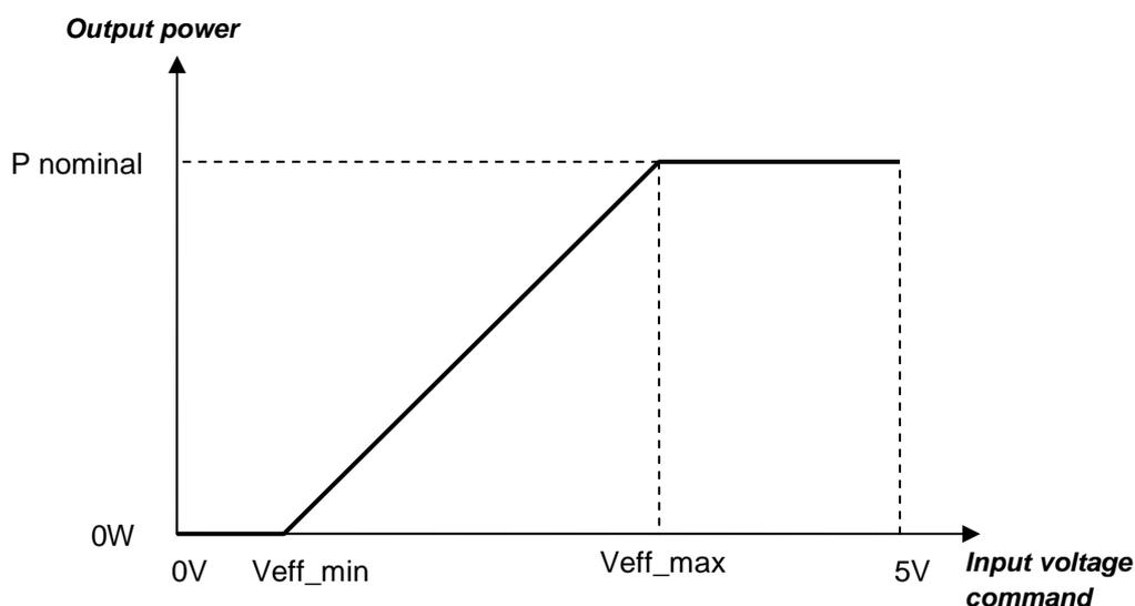
Figure 5: output power vs input voltage command typical characteristic
